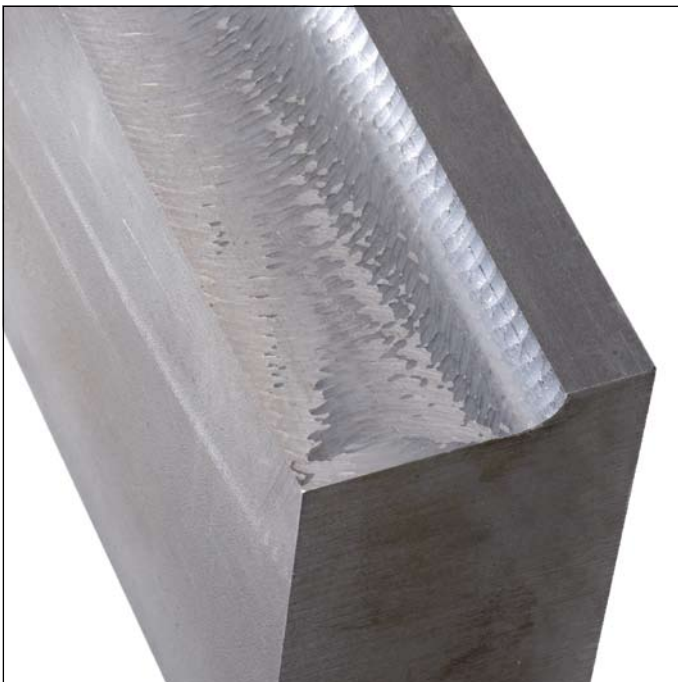
Part milled without ACC: Chatter marks are clearly visible.
